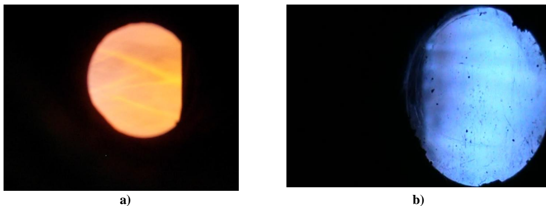
Figure 3 – The nature of the flame during the combustion of natural gas in the turbine 10 MW: (a) for standard (register) technology, (b) for MIT-technology
