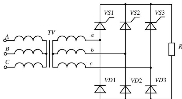
Figure 2 – Three-phase asymmetric controlled bridge rectifier
