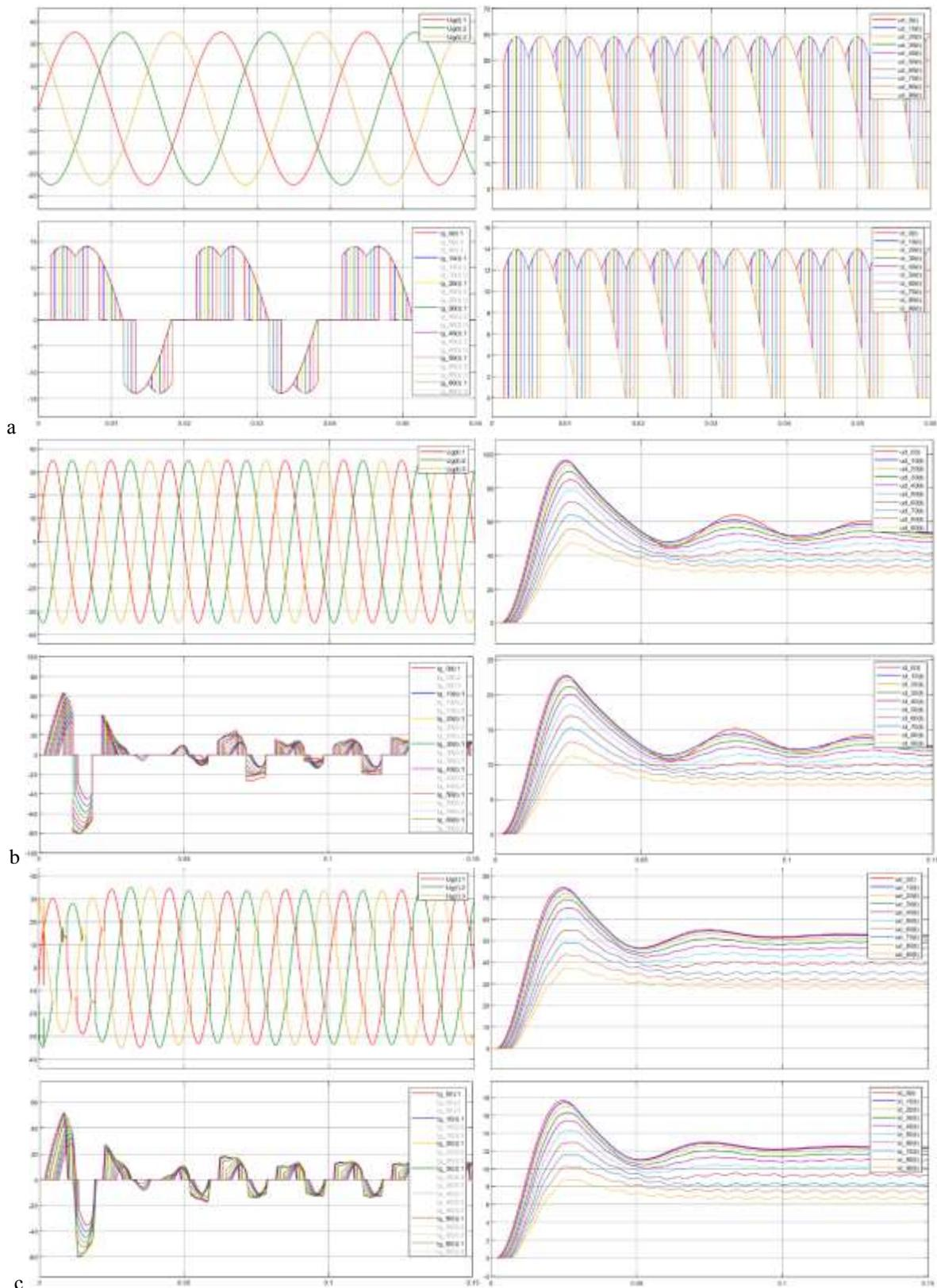
Figure 4 – Time diagrams of the network voltage ( $U_g$ ), network current ( $I_g$ ), load voltage ( $U_d$ ), and load current ( $I_d$ ) as the control angle of the thyristors ( $\alpha$ ) changes:
