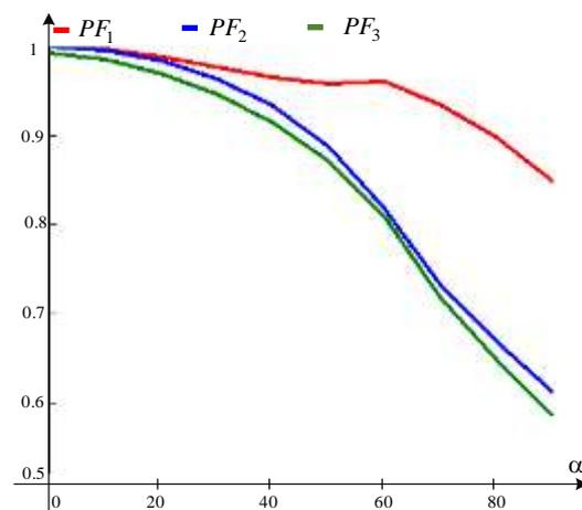
Figure 10 – Dependence of the PF value on the thyristor control angle.
