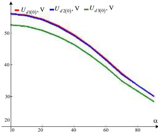
Figure 11 – Dependence of the zero harmonic value on the thyristor control angle.
