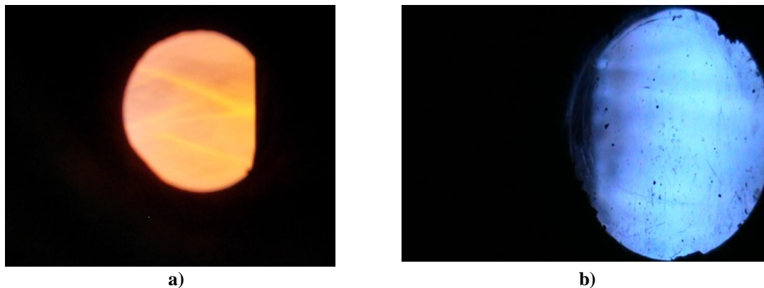
Figure 3 – The nature of the flame during the combustion of natural gas in the turbine 10 MW: (a) for standard (register) technology, (b) for MIT-technology
